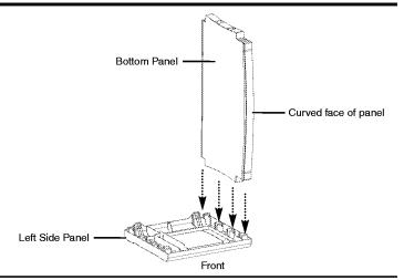
2. With the curved face of the Top Panel facing the front of unit align holes in side of Top Panel with corresponding tabs on Left Side Panel and apply pressure to snap in place.
