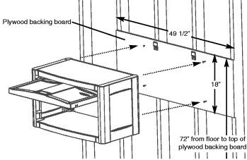
8. Metal Mounting Brackets are screwed into pilot holes using provided 2" screws
