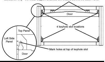
10. Push Wall Anchors into 1/4" diameter holes, making sure to push until Wall Anchor Heads are against wall. Screw two of the provided screws into the bottom Wall Anchors only.
